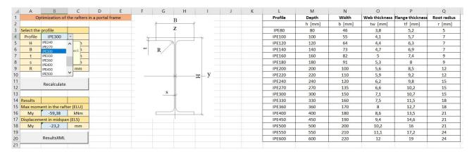
Now once we chose a profile, all the dimensions will be automatically updated in the Spreadsheet. We chose for example an IPE400: we run "Recalculate" and "ResultsXML" and we get the final result.
